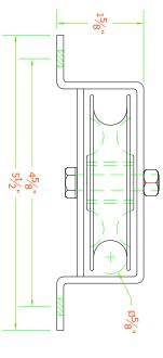
BODY MATERIAL:  $\frac{1}{8}$ " HRO STEEL WHEEL MATERIAL: REINFORCED NYLON
